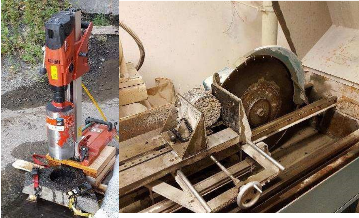
Figure 7. Asphalt and Concrete Sample Preparation using Coring Drill and Circular Diamond Saw 136
